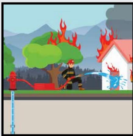
Water flowing through the system to fight the fire creates suction in the system called 'backflow.'
